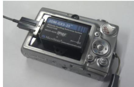
Figure 1. Microstrain 3DM-GX3 IMU attached to Canon IXUS 750 camera
