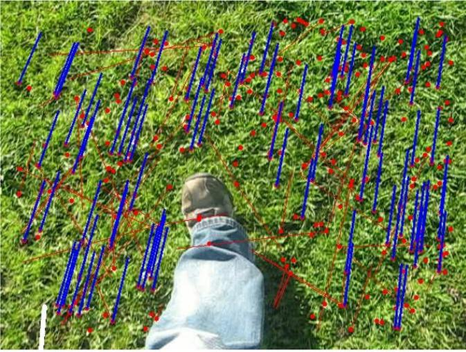
Figure 4. Features (red dots), inlier correspondences (blue lines) and outliers (red lines) marked on example frame
