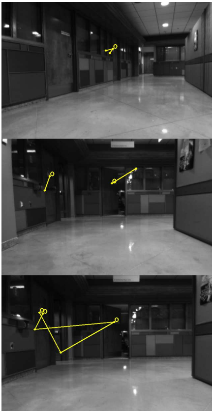
Fig. 12. BoW objects from the same class observed on several similar-looking doors, University of Alberta dataset. (Each BoW object is measured in one place per pair of frames, however in BoWSLAM each frame is registered to many others, so the same type of object may be measured in several places in the same frame.)
